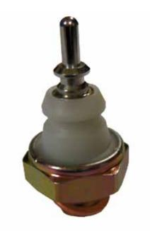
The Thermometrics Oil pressure switch monitors the engine oil flow when the engine starts. It can detect oil pressure and enables the EMS ECU to check for the lack of oil. It can also send an alarm signal to the driver, helping to avoid engine damage due to overheating.
