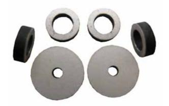
The Thermometrics Washer-Type Thermistor is used to measure the temperature of an automobile engine. The thermistor has excellent mechanical characteristics, including a bending strength of 14.7 N (minimum) and the compression strength of 9.8 N. The thermistor is heat-proof, has a wide operating temperature range and is reliable.
