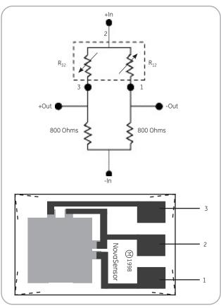
Die dimensions (I x w x h): 1150 µm x 725 µm x 190 µm, Pad Size: 200 x 150 um, Pad Material: Au *P165 schematic diagrams*
