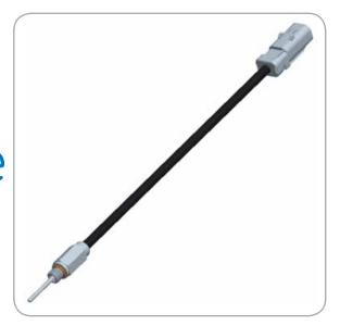
The pigtail manifold air temperature sensor measures the air temperature in the intake manifold of several sizes of diesel engines. Its function is to assist the engine control unit in engine control. This results in better fuel efficiency and lower emissions/
