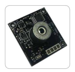
The ZTP-188ML infrared module is used for non-contact surface temperature monitoring. This thermopile IR module presents the temperature compensated 8 linear array outputs via UART with optics (Silicon Lens). It can also provide compatibility with the customer's device without the need for recalibration. The ZTP-188ML uses 4-wire connections: two signals for I<sup>2</sup>C output, single power supply and ground.
