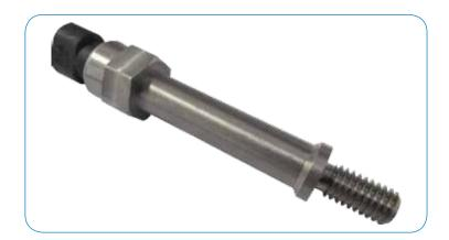
This temperature sensor monitors the temperature of an engine cylinder head. This sensors purpose is to provide a signal output that is proportional to engine temperature. This signal can be used as an input to a temperature gauge, provide input to an ECU (Engine Control Unit) or control a cooling fan circuit.
