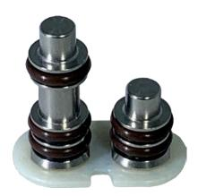
Thermometrics A-2152 Plug Detection Sensor is subjected to a specific voltage to promote heating of the sensing element. This is combined with the end user's fluid running past the sensor, which causes the sensor to cool down until a plug or loss in flow rate occurs. The sensor element will alert the system when a specific resistance is met for self-heating i.e., plug or loss in flow rate.
