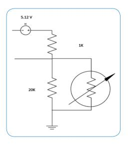
At this point, power across the NTC will be  $\sim$ 6.24 milliwatts. This will be the value needed for the power budget.
