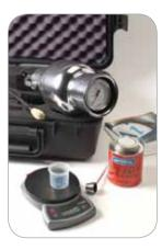
reacts with the reagent to produce a gas and pressure rise within the vessel that is proportional to the amount of moisture. The moisture content value is then read directly form the calibrated pressure gauge.
