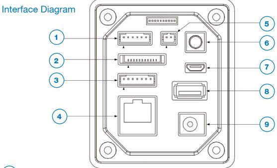
1 6-PIN Open Button, Door Check, Fire Interface
