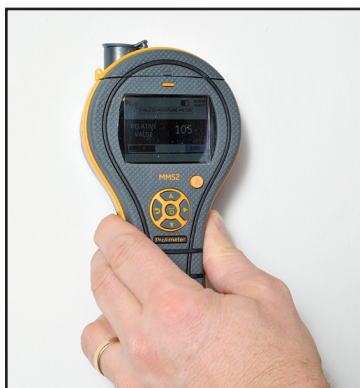
Figure 3: Taking Relative Moisture Readings
