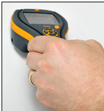
Figure 2: Using the Pin Moisture Meter
