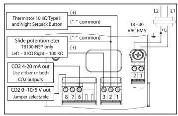
Figure 2: T8100-NS/NSP Wiring for 3-Wire System, AC Power
