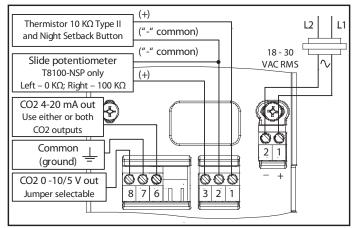
Figure 3: T8100-NS/NSP Wiring for 4-Wire System, AC Power
